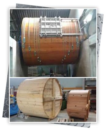
The OaC Technology is based on a concept of opening and closing of the pores of the leather that allows the products to penetrate better in it and at the same time lower the percentages of these products bringing the improvement of all the processes carried out in cask from start to finish, which is by improving opening in the initial stages of manufacturing and the final quality of the leather. This operation is carried out by the mechanics produced by the internal system of the drum.
